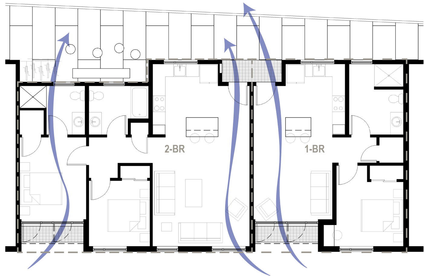
NODES - Nested unit plans allow passive cooling and a range of interior and shared social connections.
