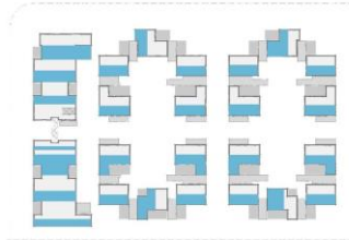
Opaque Solar Panels on all South and West Facing Roofs = 13,362 sf
